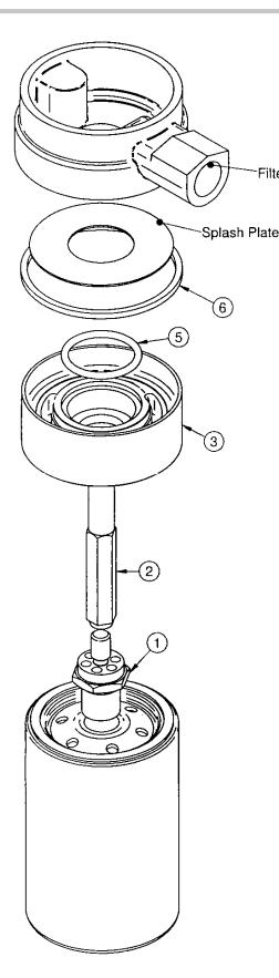
To compensate for the variations in Filter Head tolerances the Spin On consists of three parts.
