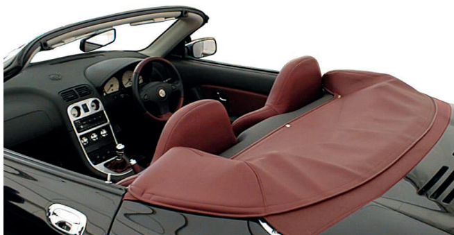
Hood roll cover, 1 press stud & 2 eyelet attachment
