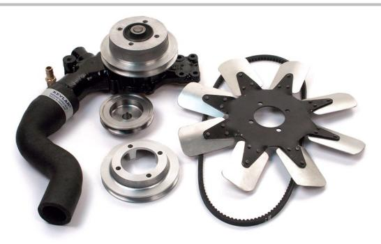
Due to the improved volume of flow created by this pump we recommend that the engine block is thoroughly washed (blasted) out, or preferably acid-dipped, as the high flow will cause any silt to eventually settle and cause a blockage at some point.
