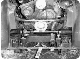
When the brackets have been tacked in place, remove the rack and finally weld the brackets to the chassis wherever they can be.
