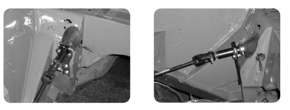
The rack can now be finally installed using bolts, washers and nyloc nuts supplied. Loosen the upper column and slide this into the cockpit slightly.
