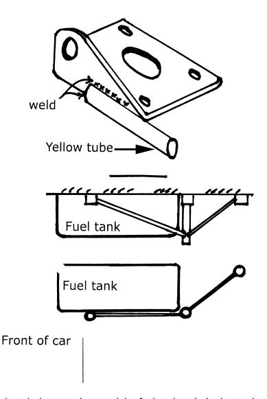
Fit the tubular tripod around the fuel tank with the long tube across the car and as close as possible to the front of the fuel tank.
