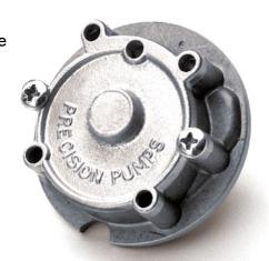
Make sure the retaining bolts do not bottom out in the relevant tapped holes in the block before securely clamping the pump to the block. Any air leaks caused by using bolts that are too long will cause oil pressure deficiencies, drain-down and oil supply problems. Do not over-tighten the retaining bolts - the torque setting is only 8-10 lb ft. Over-tightening will cause the same problems detailed above by causing the gasket to split.
