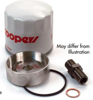
You are now ready to fit a spin-on filter to your Jaguar. Use our 011.050 high quality filter with a 3/4'' UNF thread. Remember to fill the filter with oil before fitting and change it at the recommended intervals.
